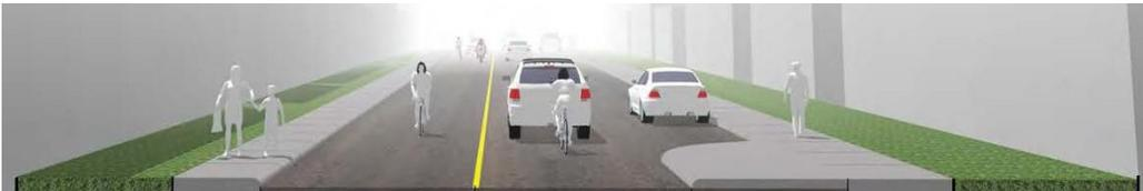
**Figure 3: Example cross-section of O'Connor Street Bikeway looking north at Patterson Avenue (cross-section varies by block; refer to functional plan) – Shared-Use Lanes**
